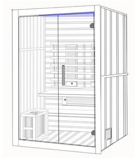
(10) Place Ceiling panel onto the installed walls
