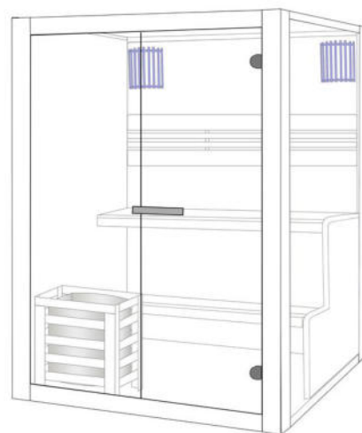
(15) Install the wooden lamps by preset hooks, and plug in the cable connectors on roof.
