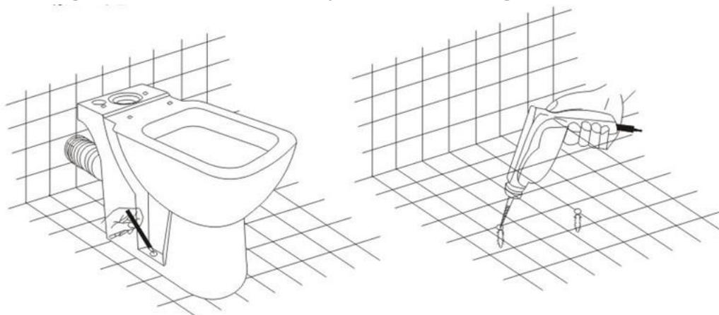
4. Toilet base will be fixed on both sides of the hole at the ground lay the fixed screw holes, install the screws, such as excessive force, ceramics have the possibility of cracking. Will then take over the base of the sewage outfall, and to connect outfall crossing, with the base to take over the sewage outfall and the outfall, crossing the junction sealed plastic glass.
