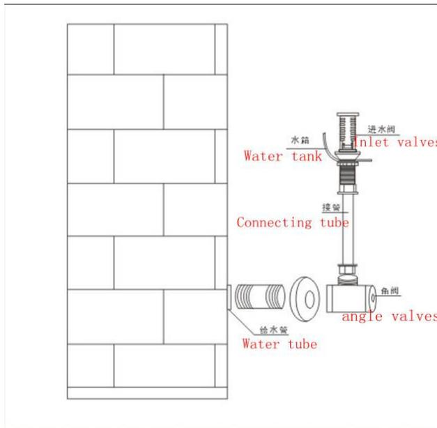
8. Angle Valves will open the water and check the tightness of the connection points small. In accordance with the installation of manual adjustments to make water into the float tank to tank water level.
