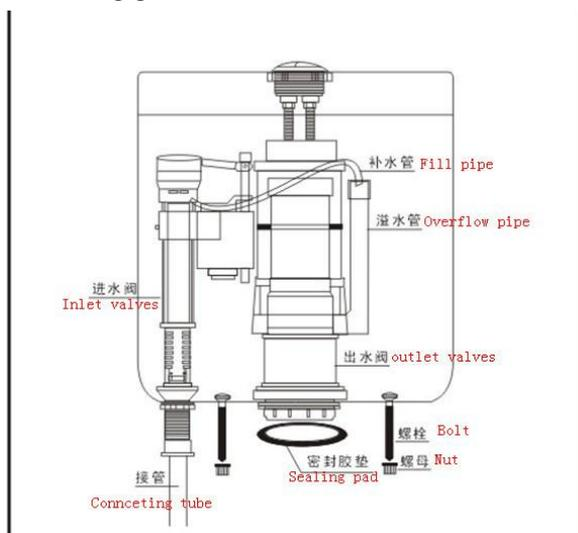
6. Accessories will be installed water tanks, sealed onto pad. Insert the bolt tanks and Toilet at the base of the mounting hole, nut tightening around the turn until the water tank installed in the Toilet solid base.
